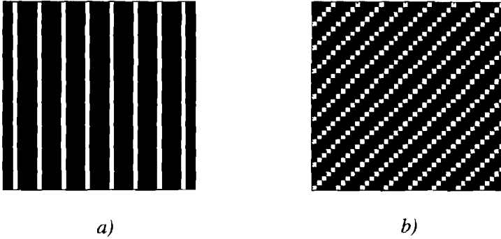
Fig 1: a) A vertical line halftone with dot gain 9.9%, b) A slanted line halftone with dot gain 11.7%.
