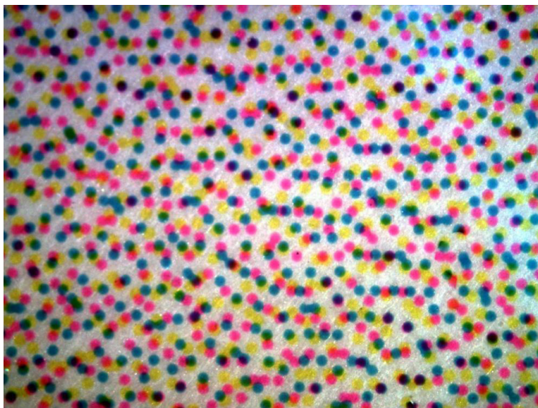
Figure 2. Photomicrograph of a 10% patch of CMY inks printed on white BOPP that has been surface-treated with polymer-dispersed divalent metal salt.
