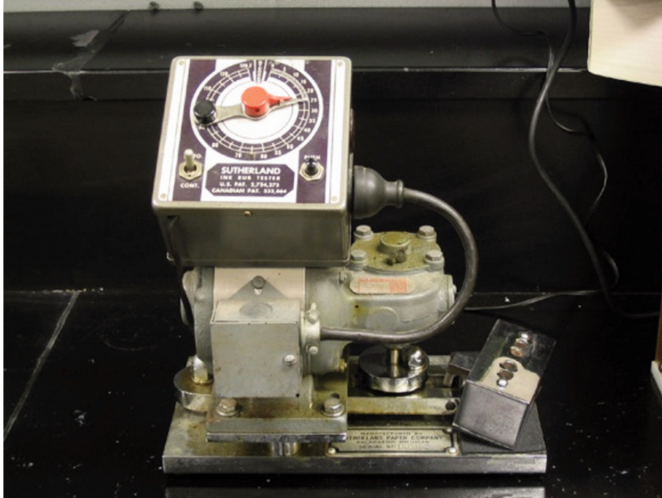
Figure 3. Sutherland Rub Tester used in this study.
