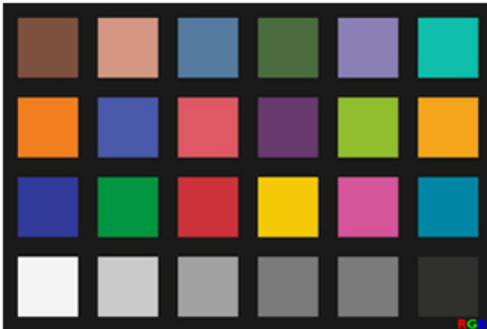
Figure 3. X-Rite Color Checker Chart used to measure color differences
