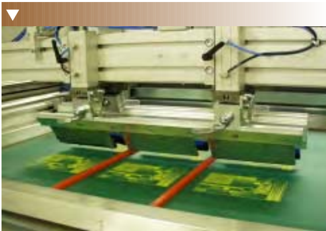
Figure 8: Square squeegee strips were glued on the screen as dividers to keep the inks separate.
