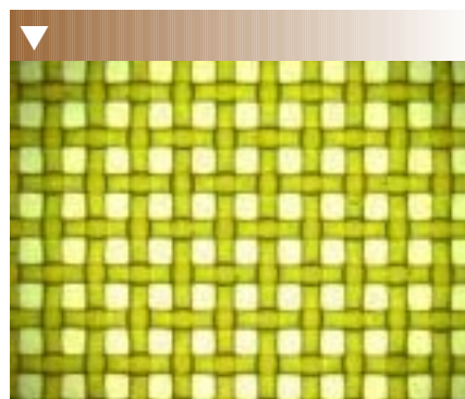
Figure 18: Image taken in the 50 percent area of Chemical 2, solvent ink, reclaim only method using 1,000 psi after the second print run reclaiming.
