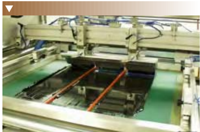
Figure 9: A sectionalized squeegee and floodbar were used to print all three inks at once.
