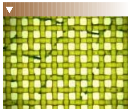
Figure 17: Image taken in the 50 percent area of Chemical 2, solvent ink, reclaim only method using a garden hose after the second print run reclaiming.
