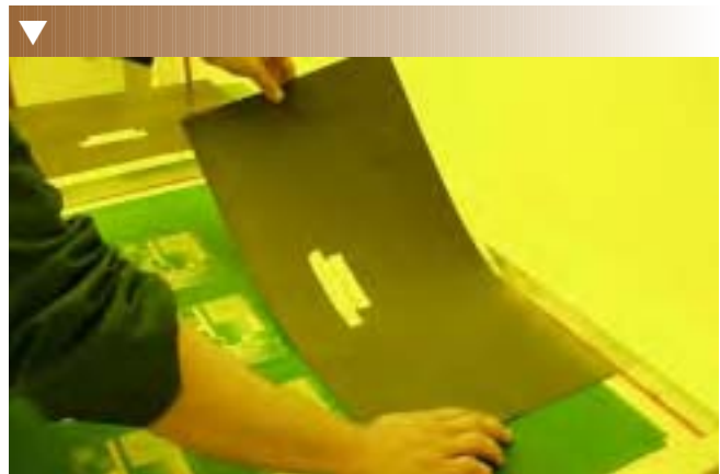
Figure 10: Magnetic sheeting on both sides of the screen was used as the first mask to cover one row.
