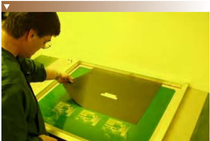
Figure 13: The second mask covered two rows, including the row the first mask protected.
