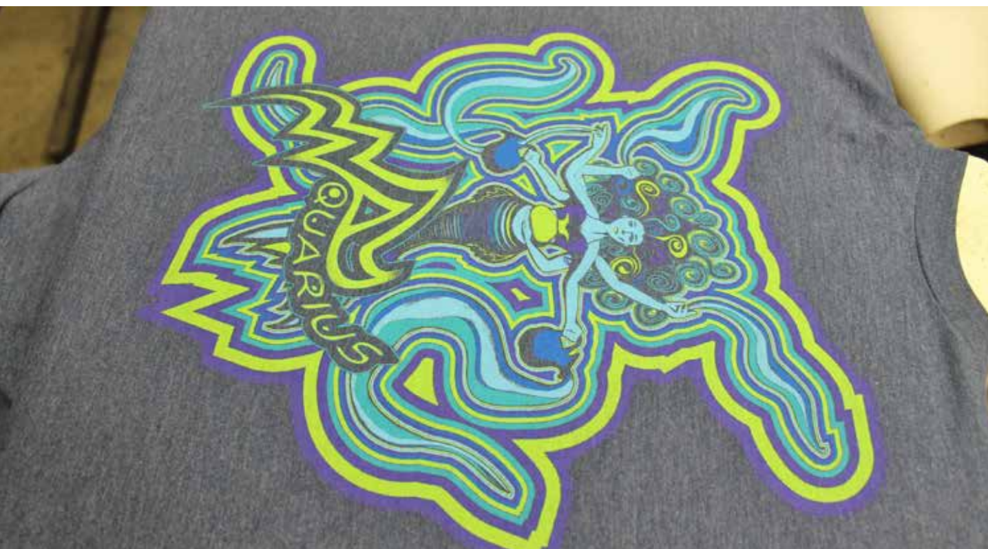
Three-color psychedelic design printed with Aquarius Bright Discharge Base ZF. All discharge colors are printed with 200 mesh and one squeegee pass for each color. (Courtesy of Jenny Ortolani.)
