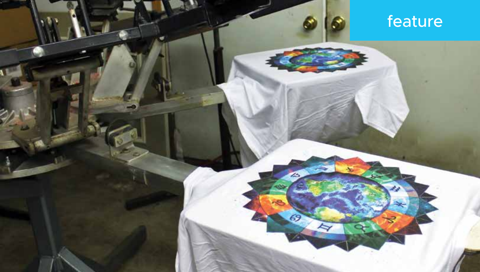
Shirts printed with Aquarius Soft Base CMYK, showing the ability to capture a wide spectrum of color with just four screens plus a white highlight screen. (Courtesy of Jenny Ortolani.)
