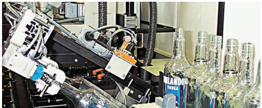
Kammann's K9-V is a universal screen-printing machine for decoration of cylindrical plastic and glass containers.
