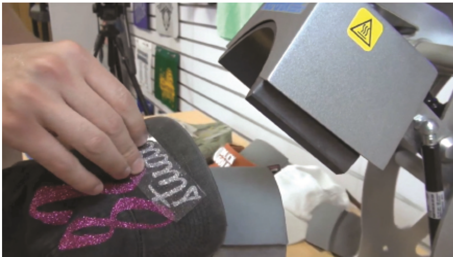
Using heat transfer vinyl and a cutter, it is a simple process to cut and weed a design that can be applied to a cap with a heat press. Photo courtesy of Stahls.
