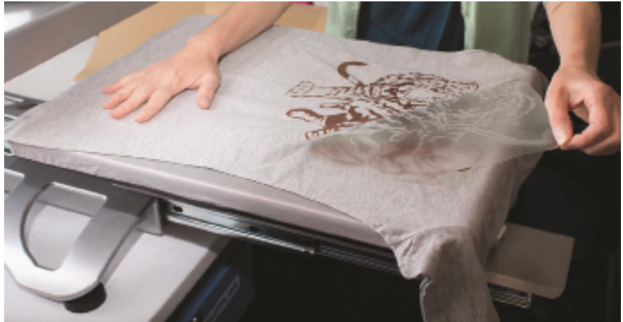
Heat-applied vinyl offers significant time savings over screen printing or embroidery. It's also ideal for small quantities. This process requires a vector file. Photo courtesy of Stahls.
