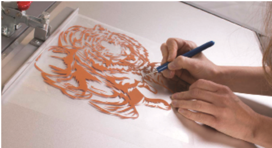
Weeding makes vinyl cutting more labor intensive than digital direct-to-garment printing or digital transfers. Once the vinyl is cut, the excess must be removed before applying the graphic to a substrate. Photo courtesy of Stahl's.
