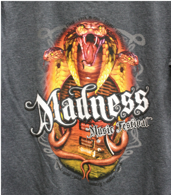
For full-color screen printed designs you can use vector or raster artwork. The artwork must then be color separated. This example is a simulated process color separation created from a raster image with vector text. Graphic courtesy of Great Dane Graphics.
