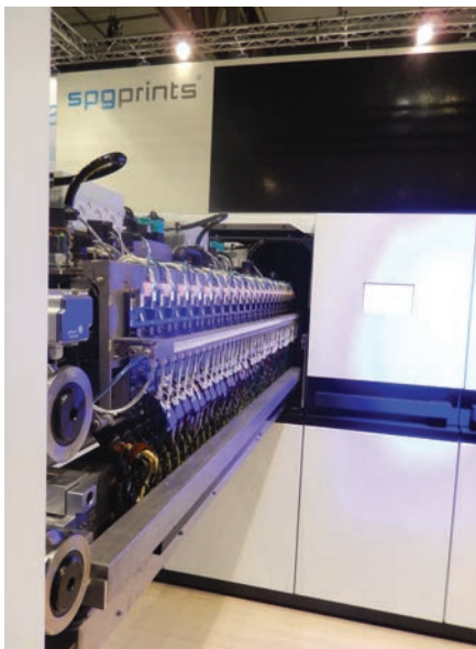
SPG Prints PIKE single pass inkjet textile printer Printbar with Fujifilm Dimatix Samba PIJ heads
