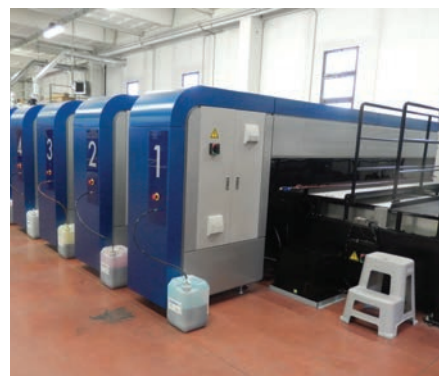
Input end view of Konica Minolta Nasseger single-pass printer
