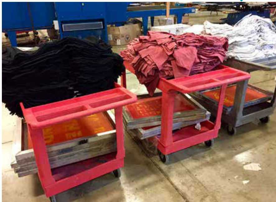
Unboxed inventory staged on carts by press with screens. These are lined up in the order they need to be produced. (Image courtesy of Atkinson Consulting.)
