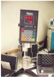
Figure 42: Digital, temperature controlled ink stirring motor/mixer with attachments (Brookfield).
