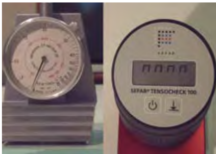
Figure 27-28: Mechanical tension meter (left) and Digital tension meter. (right).
