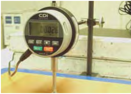
Figure 17: Digital depth gauge on comparator stand.
