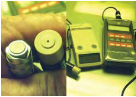
Figure 18: Digital induction screen thickness gauge.
