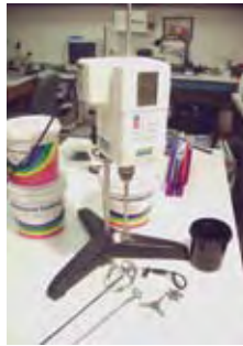
Figure 43: Programmable ink stirring motor/mixer with attachments.
