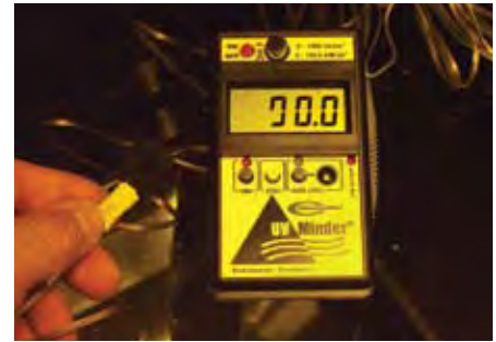
Figure 24: UV exposure radiometer and probe.
