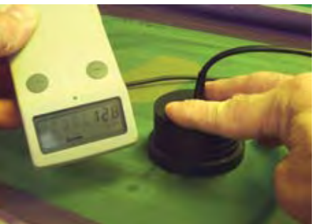
Figure 32: Inductive electronic off-contact gauge (DeFelsco).
