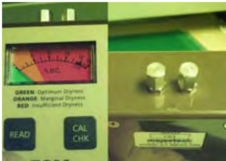
Figure 29: Inductive humidity meter (left) probe detail (right).
