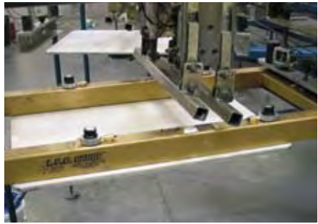
Figure 34: Dedicated head-size-specific, off-contact gauge (LOC gauge, SDI inc.).
