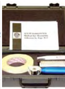
Figure 45A: ASTM certified cross-cut adhesion test kit.
