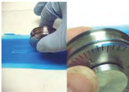
Figure 40: "Coil" or "wheel" type wet ink film thickness gauges (Gardco).
