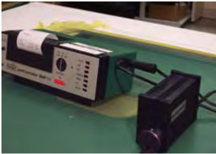
Figure 21: Bench-top perthometer and Rz meter.
