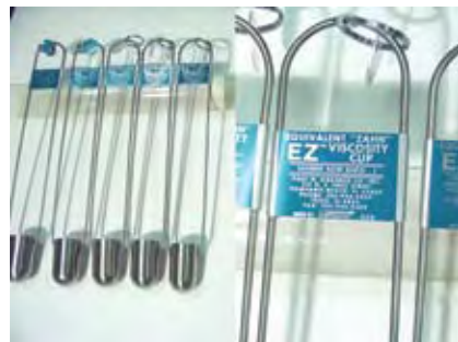
Figure 41: Zahn viscosity testing cups (Gardco).
