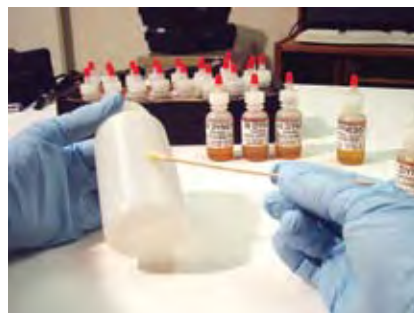
Figure 46: Dyne level test kit.
