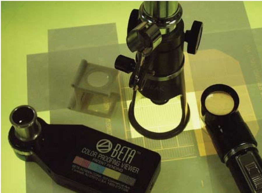
Figure 7: From the left, an 8 times magnification (8X) folding linen tester, 45X stand microscope, 12X lighted hand loupe, 20X lighted color-correcting loupe.
