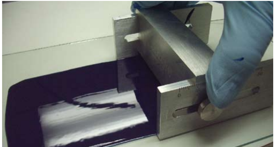
Figure 4: An adjustable-drawdown bar for ink film and color density testing.
