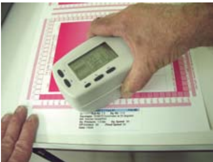
Figure 2: A reading of the hue variations with a reflectance densitometer.
