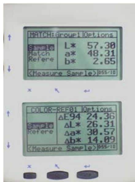
Figure 3B: Spectrodensitometer screens show LAB color mode (top) and absolute color difference mode (bottom).
