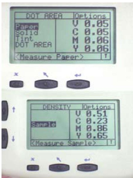
Figure 3A: Densitometer screens show dot function mode for measuring dot loss and gain, as well as half-tone percentage (top) and color-density mode (bottom).
