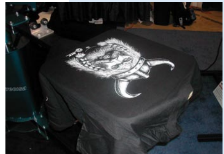
Figure 3: For this multicolor print on a dark shirt, a white underbase was first applied. This type of underbase is tonal, not a solid. You can see that instead of a solid sheet of white ink, the white is printed in varying degrees of opacity.
