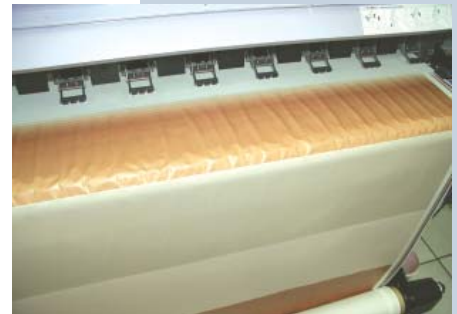
Figure 4: Alternating dark and light bands. Note the cockling at the borderline.
