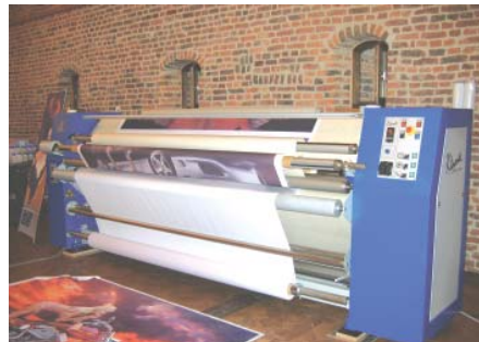
Figure 3: Roll-to-roll transfer in a transfer calender.
