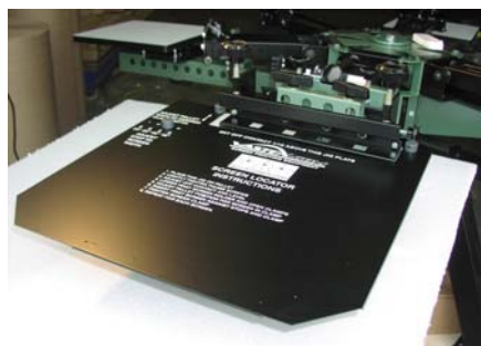
Figure 18: This specialized jig designed as part of Vastex's pin registration system, fits any Vastex standard 15-by-17 inch pallet. It can be customized for any size pallet.
