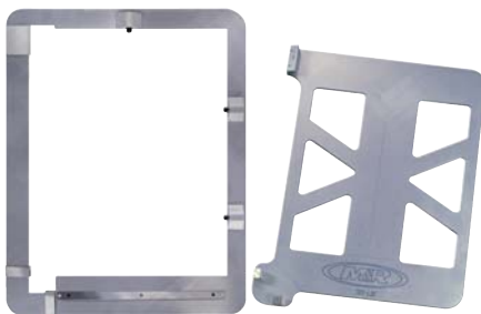
Figure 9: M&R's rapid registration system consists of a master registration frame, a registration pallet, one pin bar, stop blocks for accurate positioning of the Tri-Loc pallets and pre-punched carrier sheets. This photo shows the single frame Tri-Loc, a double-frame version also is available. Photo courtesy of M&R.
