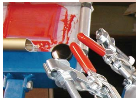
Figure 4: For the budget-minded, R Jennings offers free instructions on how to construct your own pin registration system. It supplies the pins, a drill fixture and special clamps. The company also will install the pins on your clamps if you want to ship them to the facility. Photo courtesy of R Jennings.
