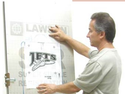
Figure 5: Position your positive on the vacuum alignment board. Put double-sided tape on the positive and turn on the vacuum to hold it in place. Photo courtesy of Lawson Screen Products.
