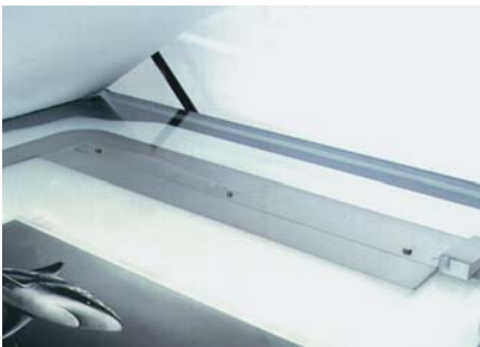
Figure 10: The Tri-Loc master registration frame is mounted directly into the exposure unit. Film positives are mounted on a carrier sheet, then placed on a pin bar positioned on the master registration frame. Photo courtesy of M&R.
