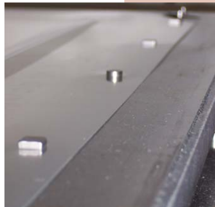
Figure 3: A pin registration system uses pins to keep artwork aligned through the screen printing process. This photo shows a pin bar attached to the mesh side of a Newman Roller Frame. Photo courtesy of Stretch Devices.
