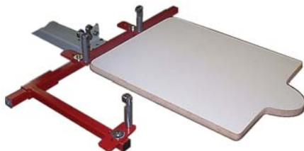
Figure 8: For instant positioning without pins, use the speed registration attachment that provides three points for your screens while you clamp them in place. It works on manual or automatic presses. Photo courtesy of Lawson Screen Products.
