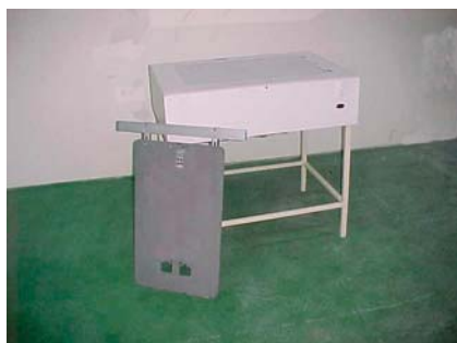
Figure 17: Figure 17: The EZY REG system offered by TAS America includes a light box with a layout grid, an oversized pallet, a pin or a non-pin alignment fixture, and carrier sheets. It works on only specific TAS models and is compatible with rigid and retensionable frames. Photo courtesy of Tas America.
