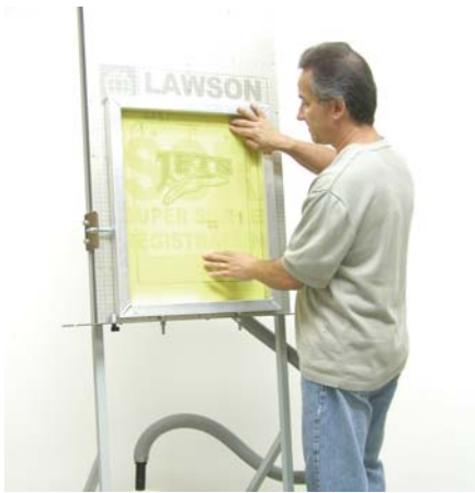
Figure 6: Place your screen in position resting it at the bottom of the alignment board on pins. Press the screen against the tape. Photo courtesy of Lawson Screen Products.
