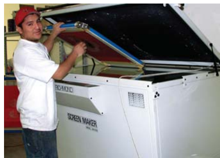
Figure 2: Some printers mount a pin bar on their exposure unit to speed up registration and ensure greater accuracy. According to Mark Coudray, Coudray Graphic Technologies, “It can be done on the exposure unit or off depending on whose system you are using.”
