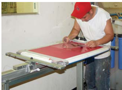
Figure 1: Many printers use the eyeball method when registering film positives on their screens. While this method works fine in many cases, using a registration system offers greater accuracy, consistency and can significantly speed up the process.
