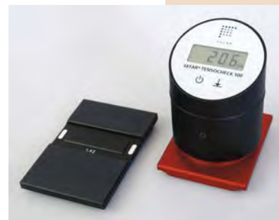
Figure 5: A modern digital tension measuring instrument: the SEFAR Tensocheck 100 with its calibration plate (Illustration to be adapted)
