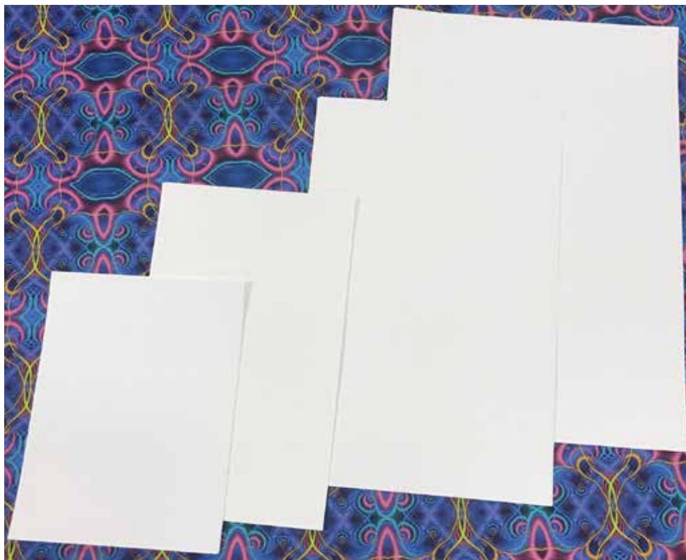
Desktop and small-format dye sublimation papers are clay (solid surface) coated to allow for the widest range of possible applications.
