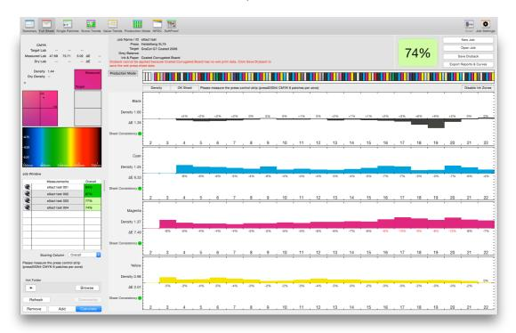
For offset printing processes it is recommended that, once the process inks are an acceptable  $\Delta E$ , the RGB overprints also be checked for Trapping % and  $\Delta E$ . If they are out of tolerance then adjustments to press settings or consumables may be required, which can affect the plate compensation required to achieve the neutral print density curve.
