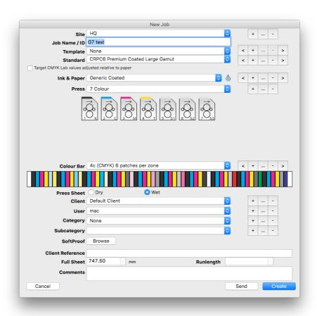
The standard chosen reflects the desired solid and overprint colour targets and how the print is to be scored. If you have not already done so, please refer to **Chapter 8 - Adding Press Targets** starting on page 29 of the QualityPass Manual, for details of how to setup a GraCol G7 standard.
