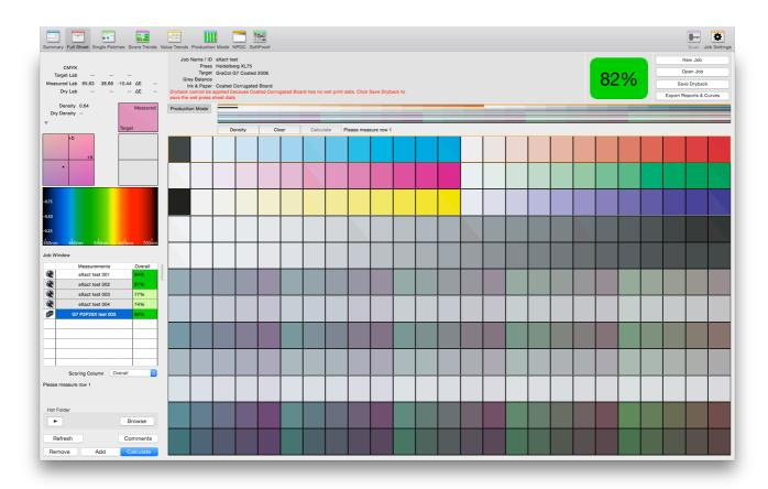
Start with line 1 and measure sequentially. The software automatically selects the next line after each scan. The "active" line to be measured is highlighted with an orange border.
