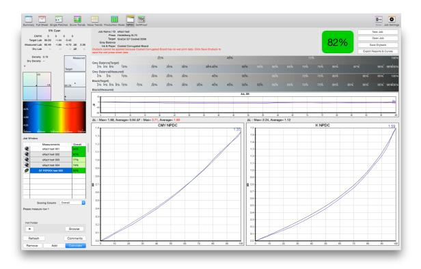
Along the top a target and measured tint ramp, for both grey balance and single black, allow a visual assessment of the colour change from 0% to 100%.
